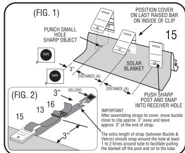
STEP 6: Assemble Cover Clip (15) as shown in drawing (FIG.1) to the pool cover equally spaced as per drawing lin previous page (SEE STEP 4 & 5). Assemble and attach Cover Strap (13) with Buckle (16) to attached Cover Clip (FIG. 2).
