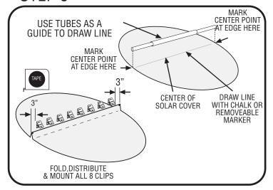
**STEP 5:** Using assembled tubes as a guide draw a centerline in the solar cover from edge to edge. Use this as a guide to attach 8 clips (15) evenly.
