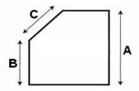
**If your spa has only 1 Cut-Corner**, begin by determining the overall length (A) and the length of the straight demension (B). Next, subtract the straight demension (B) from the overall length (A) and multiply that by 1.41 This is the length of your cut. (Rounding is OK)
