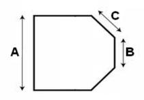
**If your spa has 2 Cut-Corners**, begin by determining the overall length (A) and the length of the straight demension (B.) Next, subtract the straight demension (B) from the overall length (A) then divide this by 2 (since there are 2 corners) and multiply this number by 1.41 This is the length of each cut (Rounding is OK)
