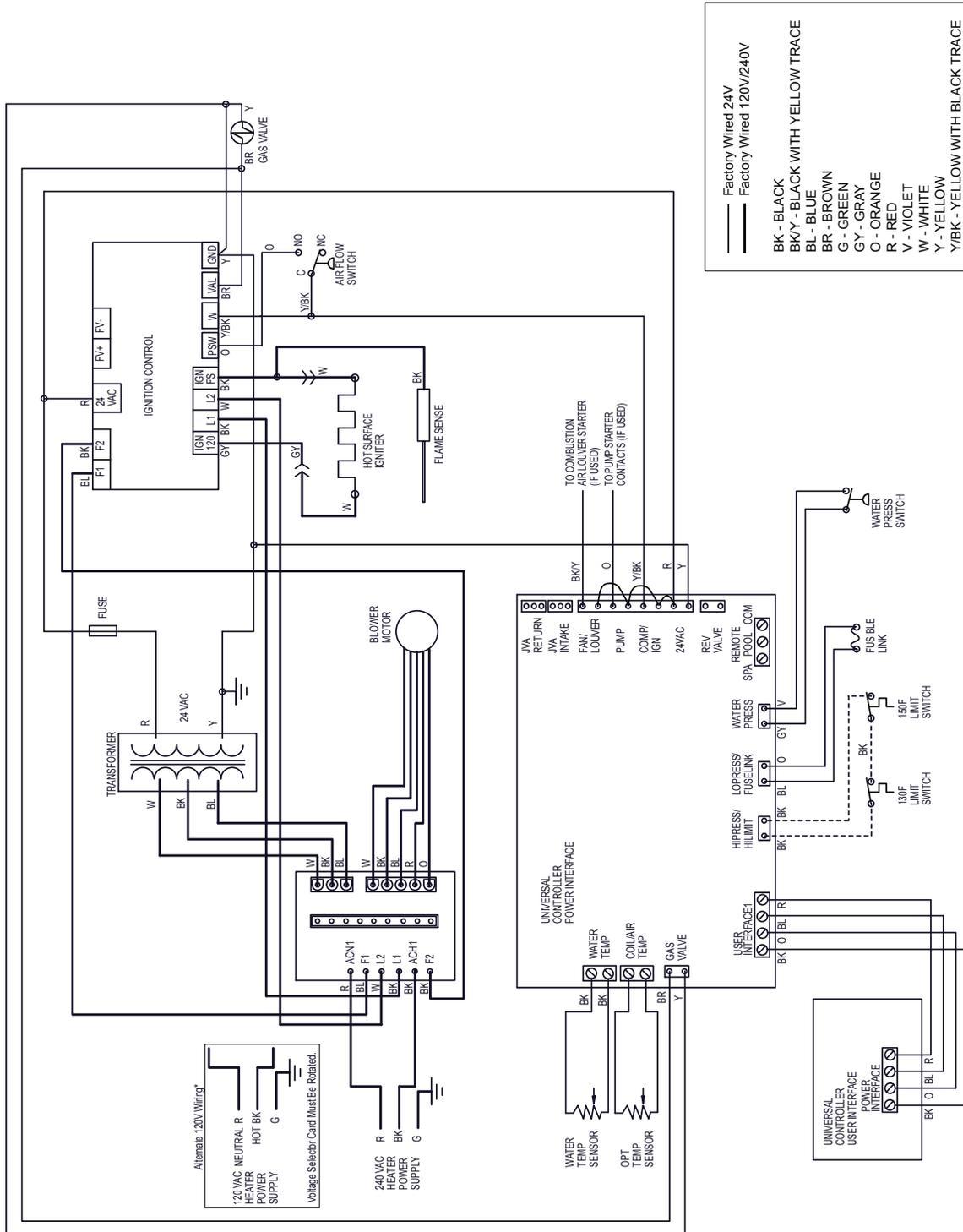
NOTES: IF ANY OF THE ORIGINAL WIRE AS SUPPLIED WITH THE HEATER MUST BE REPLACED, APPLIANCE WIRING MATERIAL RATED FOR 105°C MUST BE USED. WHERE MARKED THUS - - - - - APPLIANCE WIRING MATERIAL RATED FOR 200°C MUST BE USED. \* See Section 6.2. for Complete Details.
