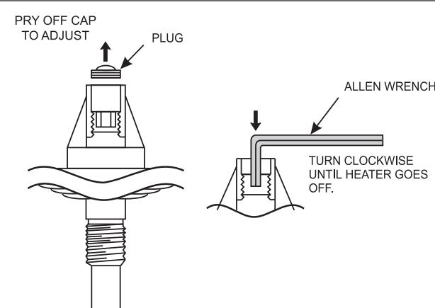
**Figure 31. Adjustment of Pressure Switch**
