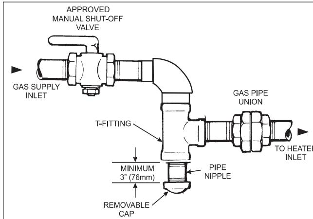
**Figure 9. Proper Design for a Sediment Trap/Drip Leg**
