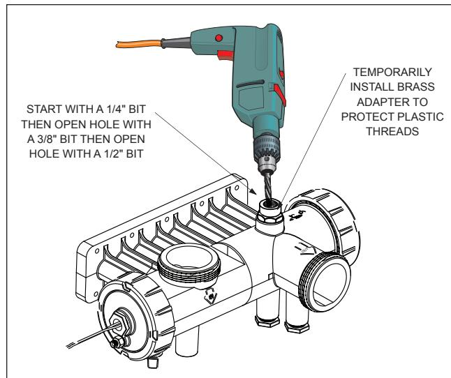
**Figure 18. Drill Hole for Pressure Relief Valve**
