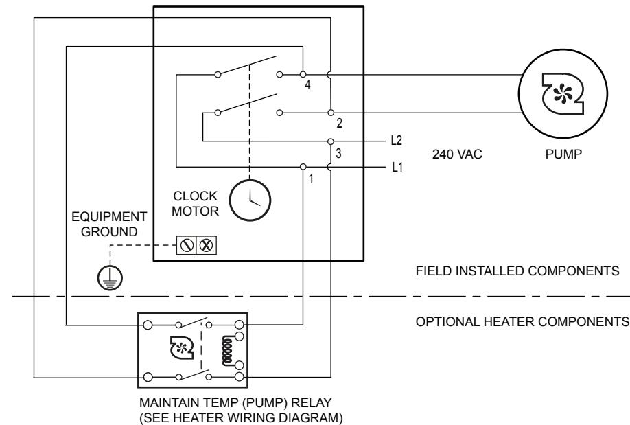
**NOTE:** INTERMATIC MODEL T104 (NOT PROVIDED WITH HEATER) WIRE CONNECTIONS SHOWN AS AN EXAMPLE, OTHER MODELS MAY HAVE DIFFERENT CONNECTIONS. CONSULT TIMER MANUFACTURER FOR PROPER CONNECTIONS.
